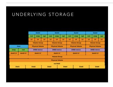
A DRBD device is generated for each one of the VMs at dom0 level. These devices have each one a domU logical volume as their storage. On top of the DRBD solution, a physical volume is created. On top of that physical volume three logical volumes are created, one for swap, one for root and another for replicated. Guests (domU) only see the DRBD as their storage, therefore only a physical volume with three logical volumes.
